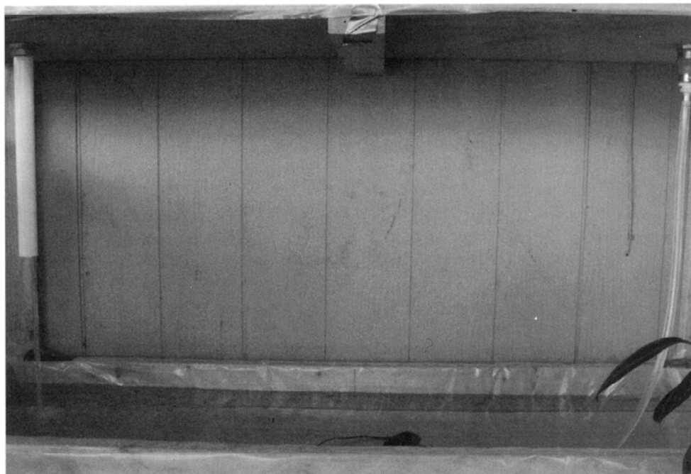
Reservoir water return pipe (left) and water delivery hose (right).
