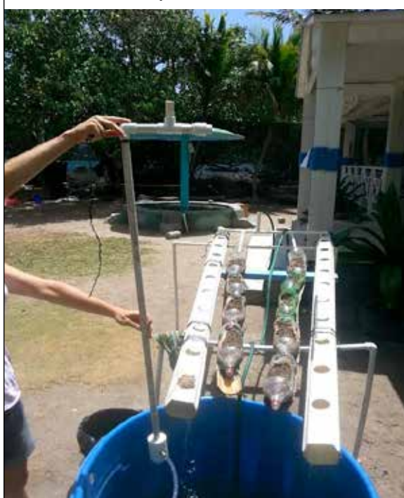
FIGURE 4.42 Simple water airlift
