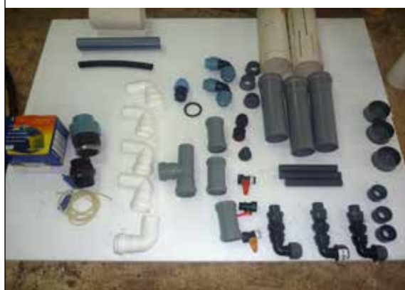
FIGURE 4.48 A selection of commonly used plumbing materials
