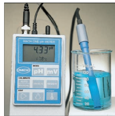
FIGURE 7.3 A pH meter can rapidly and accurately measure the pH of an aqueous solution.
