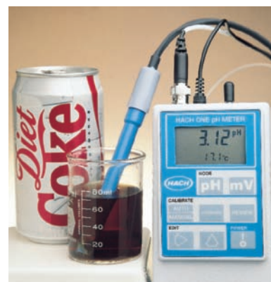
The pH of this soft drink is 3.12. Soft drinks are often quite acidic.
