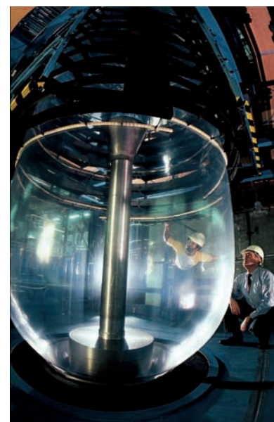
Polyethylene films are produced by extruding molten plastic through a ring-like gap and inflating the film into a balloon.
