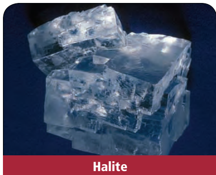
■ Figure 8 Halite has perfect cleavage in three directions; it breaks apart into pieces that have 90° angles. The strong bonds in quartz prevent cleavage from forming. Conchoidal fractures are characteristic of microcrystalline minerals such as flint.
