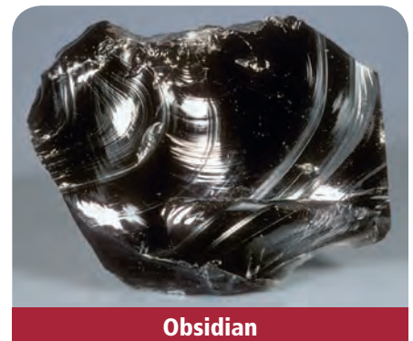
■ Figure 10 Rhyolite, granite, and obsidian have different textures because they formed in different ways. Obsidian's glassy texture is a result of rapid cooling.
