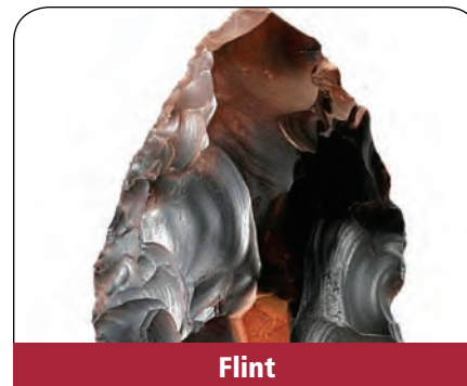
■ Figure 8 Halite has perfect cleavage in three directions; it breaks apart into pieces that have 90° angles. The strong bonds in quartz prevent cleavage from forming. Conchoidal fractures are characteristic of microcrystalline minerals such as flint.
