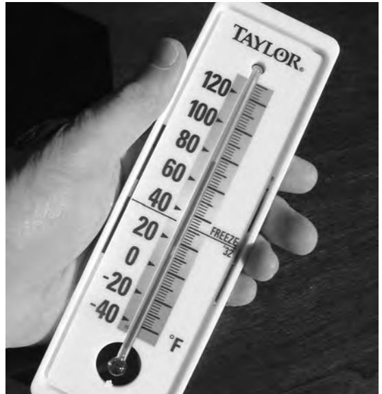
Figure 19-2 A thermometer contains colored alcohol in a glass bulb at its bottom. The alcohol expands or contracts in the tube, registering changes in temperature.
