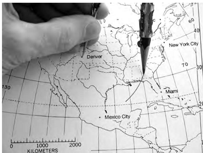
Figure 7-12 Place the point of the compass at the recording station and draw a circle at the epicenter distance. The epicenter must be somewhere on this circle.
