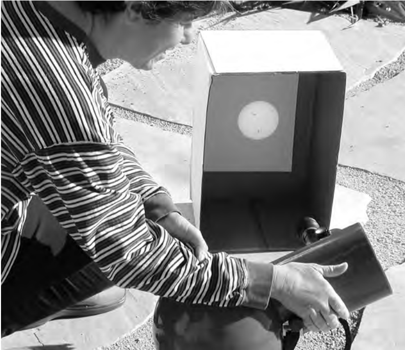
Figure 25-6 A reflecting telescope can be used to project the sun's image onto a sheet of paper mounted in a cardboard box. Dark areas known as sunspots can sometimes be seen on the sun's surface. Never look directly at the sun through any optical device.
