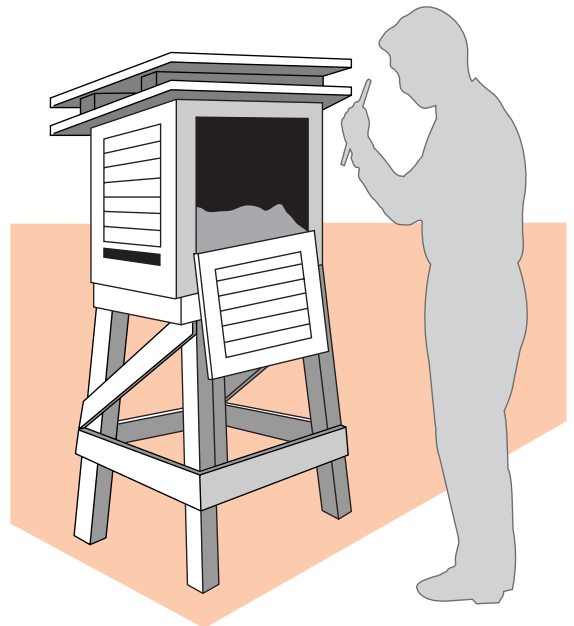
Figure 19-11 Official measurements of temperature and humidity are usually taken in a weather shelter. The shelter protects the instruments from direct sunlight; the openings in the shelter allow air to circulate.
