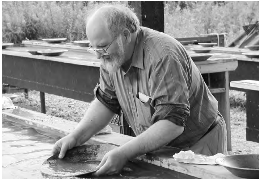
Figure 4-11 Because of its high density, gold settles to the bottom of the pan as the lighter minerals are washed away.
