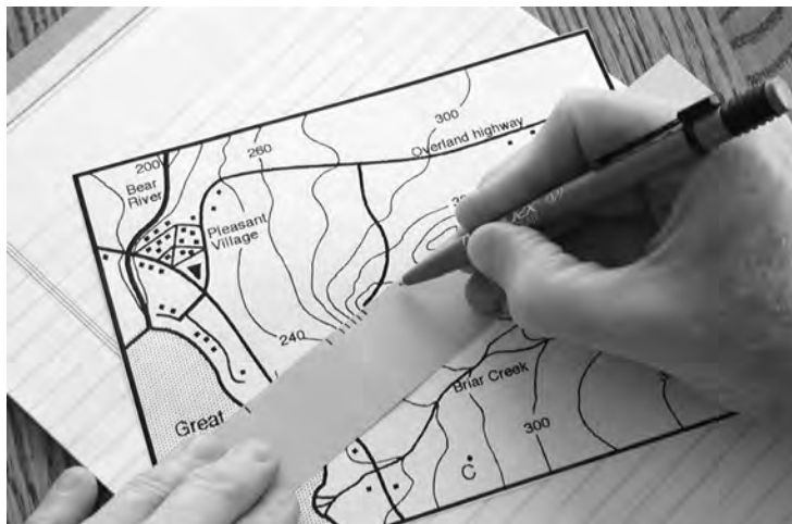
Figure 3-13 The first step in making a profile from a contour map is marking the blank strip where it crosses each contour line.
